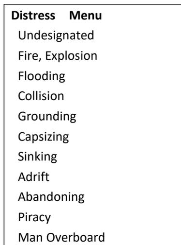
Choose one distress item such as "sinking", press and hold this for more than 3 seconds for transmitting sinking message out.
