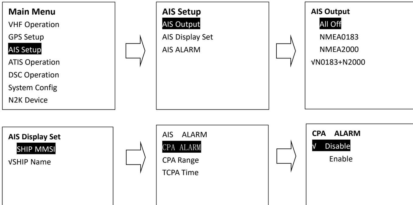
CPA Alarm enable Choose "Disable" or "Enable" item to enter disable or enable AIS alarm, then press "ENTER" key to confirm.
