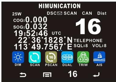
Click "Start" to activate the scan function which is searching for currently all working channels. All scanning: CH1-CH2-CH3-...-CH88. Memory scanning: M1 – M2 – M3 - ...M10 – M1- ...
