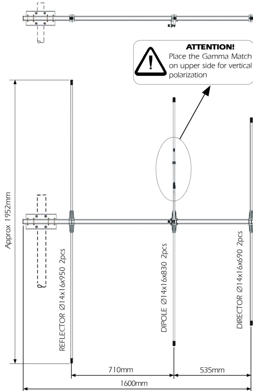
Correct mounting for vertical polarization
