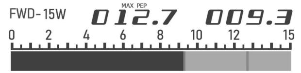
The first digit displays the maximum RF power, and the second data displays the instantaneous power. The following progress bar
