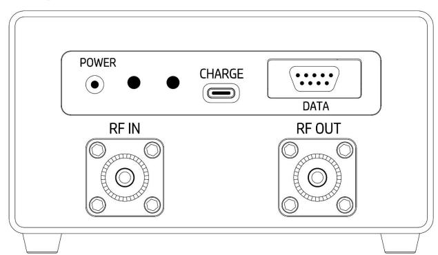
RF IN RF signal input. Connect the transmitter or amplifier.
