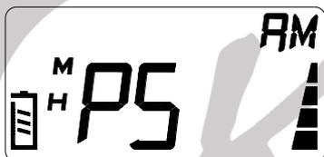
With the **[down]** and **[up]** buttons you can select the 'battery power save' level. There are four battery power levels: off / 0-4. Press the **[F]** button to store the new settings and to go to the next function. To go back to the operation mode after storing the new settings press the **[PTT]** button.
