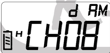
Press the **[P]** button for approximately 3 seconds to de-activate the 'dual watch' function. The 'd' and
