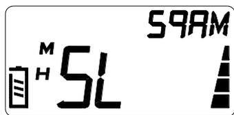
With the **[down]** and **[up]** buttons you can select the 'squelch' level. There are six squelch levels: off / 0-6. Press the **[F]** button to store the new settings and to go to the next function. To go back to the operation mode after storing the new settings press the **[PTT]** button.
