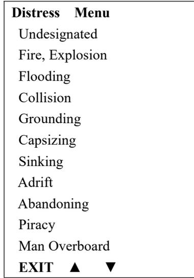
Choose one distress item such as “sinking”, press and hold this for more than 3 seconds for transmitting sinking message out.
