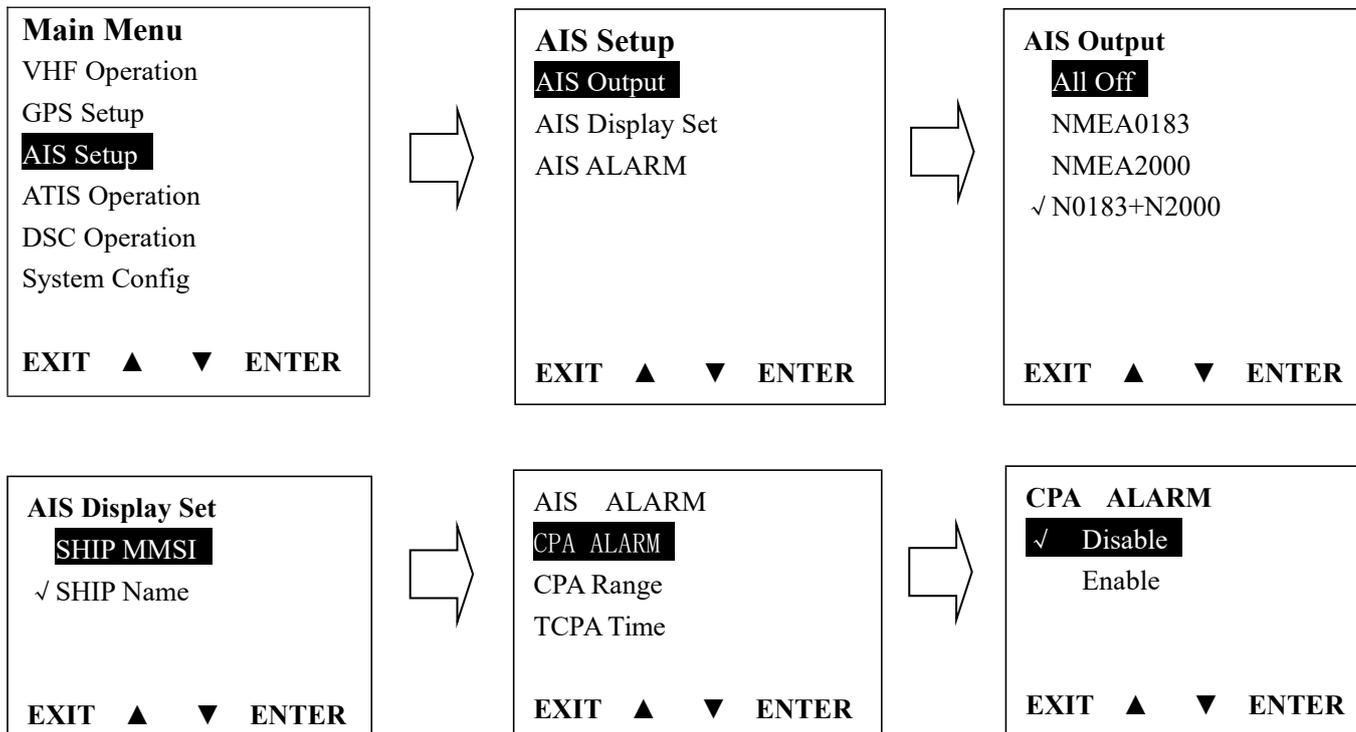
CPA Alarm enable Choose “Disable” or “Enable” item to enter disable or enable AIS alarm, then press “ENTER” key to confirm.
