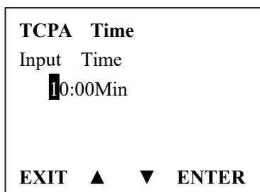
TCPA (Time closest point of approach)Alarm distance setup Press UP/DOWN key to input digital one by one, after you have done this, press “ENTER” key to confirm, the maximum input range is 30 minutes, if the input value is over than 30 minutes, the input is invalid, then the system will ask for re-enter, the default CPA value is 10:00 Min.
