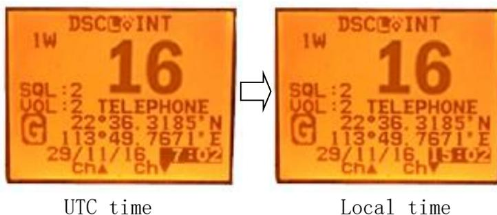
When HM390-BB cannot receive the GPS signal to display the current position, screen will automatic display the time and date. When radio received the GPS signal, screen will show the current GPS location, related UTC time and date will be shown below the GPS location mark.
