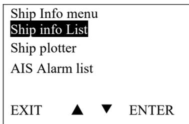
From the AIS ship info menu, you have three options: List mode, plotter mode, AIS Alarm list alarm list mode. If you choose option ‘AIS ship info list’ and press ‘enter’, you will open the list mode.
