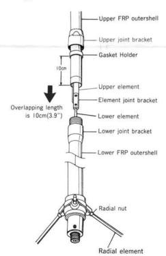
2) Put lower element into element joint bracket thoroughly and fix it.
