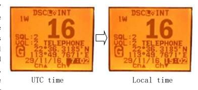
When HM390 cannot receive the GPS signal to display the current position, screen will automatic display the time and date. When radio received the GPS signal, screen will show the current GPS location, related UTC time and date will be shown below the GPS location mark.
